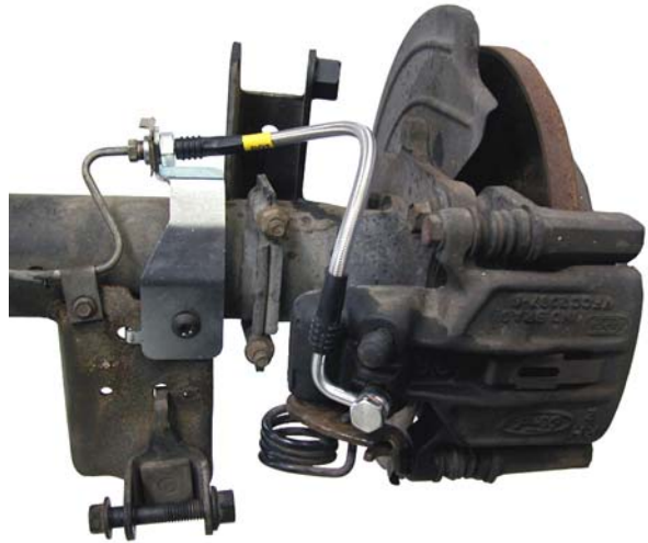
Attach new brake hose to caliper
