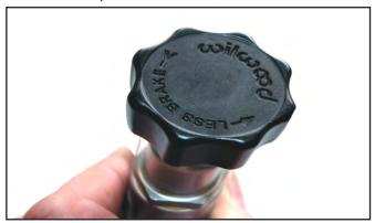
NOTE: Even at full "increase" on the knob the rear line pressure will still be slightly lower than the front line pressure. It is impossible to have higher pressure in the rear lines than the front lines with this valve.
