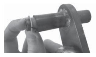
24. Locate the second, lower pair of mounting holes in the OEM pedal box. These holes are located about 1" below the original pivot holes.
