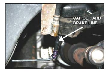
22. Unbolt the OE brake hose mount attached to the frame rail. Save the bolt for Step 40.
