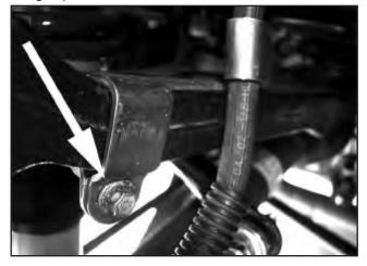
24. Unbolt the two (2) caliper mounting bolts. Save the mounting bolts for Step 26.
