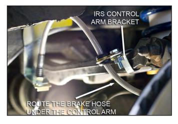
NOTE: Mounting the metal brake hose mount parallel to the control arm with the brake hose on the inboard side should provide adequate clearance to prevent the brake hose from contacting anything.
