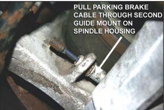
20. Use zip ties to secure the cable out of the way, or remove the parking brake cable altogether. Consult a service manual for the proper removal procedure.
