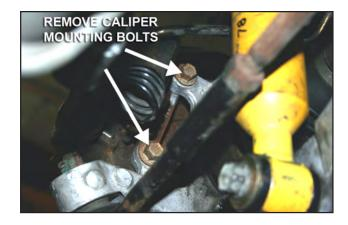
25. Remove the rotor and caliper, along with the OE rubber brake hose and frame rail bracket, as one assembly.
