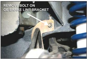
23. For 2003-2004 Mustang Cobras, unbolt and remove the brake hose locator brackets from the upper control arm. It will be necessary to spread the bracket legs apart to remove the bracket.
