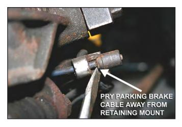
17. Remove the parking brake cable retaining clip.
