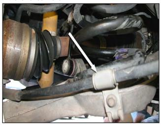
19. Pull the parking brake cable out of its spindle mount and guide hole.
