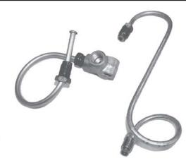
Thank you for purchasing the Maximum Motorsports 1993 Cobra/1994 GT master cylinder adapter kit. This kit allows the use of the 2 port master cylinder on 1987-93 Mustangs originally equipped with a 3 port master cylinder. The MMBAK-3 kit uses only high pressure rated fittings and adapters that are designed for use in automotive brake systems. No cutting or flaring of brake lines is needed with the MMBAK-3 kit.
