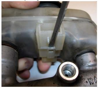
Install the low fluid level sensor into the new master cylinder by pressing in until it clicks into place.
