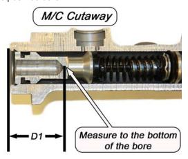
10. Measure the depth to the mounting pad and record this dimension as D2.
