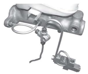
18. Install the original front port brake line and firmly tighten the two brake line fittings with a flare wrench. You may need to bend the brake line slightly to attach the fittings.
