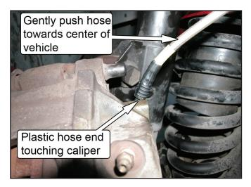
11. Torque the fluid bolt at the caliper to 14 ft-lb while gently pushing the brake hose toward the center of the car with two fingers to keep it from rotating.
