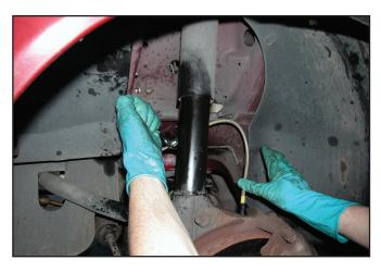
13. Temporarily remount the wheels; checking clearances to ensure the hose will not contact the tire. Have a helper turn the steering wheel from lock to lock. If it does rub, the tire *will* wear through the hose.
