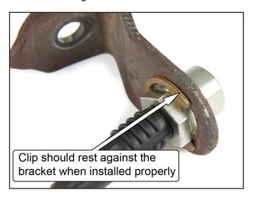
NOTE: For 1979-86 and 1987-93 4 cylinder vehicles, the hole in the bracket must be enlarged to accommodate the brake hose.
