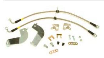
These Maximum Motorsports DOT approved braided stainless steel Teflon-lined brake hoses surpass the quality, fit, and finish of anything else in the Mustang aftermarket industry. These hoses provide better performance because their Teflon lining does not expand under pressure like a typical rubber line will. Installing stainless steel hoses will provide quicker braking response, improved modulation and a firmer brake pedal.
