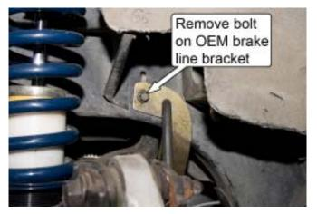
For 2003-2004 Mustang Cobra, unbolt and remove the rear upper control arm brake hose bracket from the control arm. Use a flat-blade screw driver or pliers to help spread the bracket legs apart enough to remove it from the control arm.
