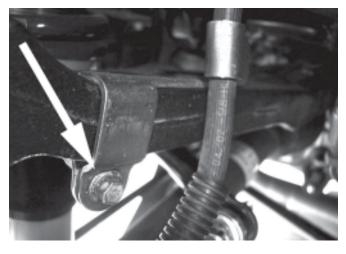
Disconnect the OEM brake hose from the brake caliper. Use a 10mm wrench or socket to remove the stock fluid bolt.
