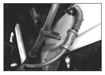
4. Unbolt the stock retainer bracket from the strut body.
