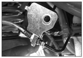
13. Using one of the supplied zip ties and rubber spacers, slide the spacer onto the tie. Loop the tie around the ABS wire at the rubber grommet, then slide the zip tie back through the spacer.
