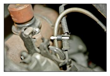
15. Snap the ABS wire into place in the frame rail mounting bracket.
