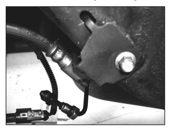
5. Disconnect the fluid bolt at the brake caliper.
