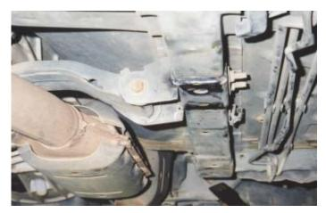
After welding the subframe connectors in place, weld the transmision mounts to the subframe connectors. Full length (MMFL-3) subrame connector is shown in the picture below. Standard length subframe connectors attach similarly.
