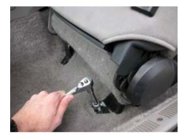
Install the supplied longer 10mm bolts with a washer under each head.  Bolt on the passenger side subframe connector. Use the included 10mm Nylock nut and 3/8" G8 washers.
