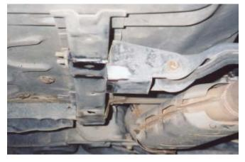
Weld transmission mount to subframe before installing subframe connector
