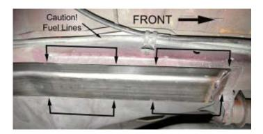
10. Weld the rear of the subframe connector to the subframe. Weld between the arrows, on *both* the inner and outer sides, as indicated in the picture below. *Do not* weld across the front end cap.
