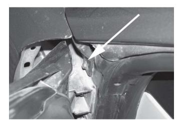
11. DO NOT remove the applique. Gently move it away just enough to open a small gap for removal of the plastic cowl at the base of the windshield.
