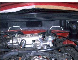
Remove the alarm siren (if so equipped) from the firewall. Then remove the plastic cover from the firewall. It is held on with several small sheet metal screws, as well as the hood seal.
