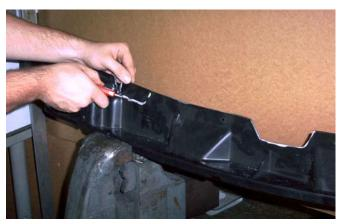
8. Put the plastic back into position on the firewall. Set the Strut Tower Brace back into position and check that the plastic is notched correctly.
