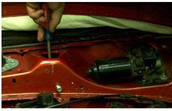
27. Install the #8 sheet metal screw into the small hole in the nutplate. Remove the 5/16"-18 bolts.
