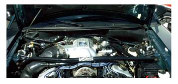
NOTE: Access to the fuse box -- the cover can still be opened by pulling the cover foward and past the strut brace main tube as you lift the cover.
