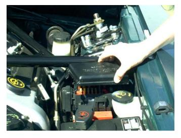
NOTE: If the fuse box cover cannot be opened, reposition the fuse box by moving it forward. This can easily be done by slipping a screwdriver between the front of the strut tower and the rear of the metal fuse box mounting tabs (these are attached to the strut tower). Gently pry the tabs forward. This will move the fuse box slightly forward.
