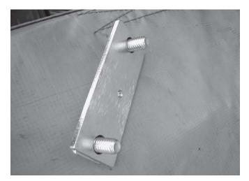
19. Line up the nutplate on the 5/16" holes drilled in the firewall in Step 19. Use the bolts installed in the previous step as guide pins. Make sure that the small hole in the plate is biased downward.
