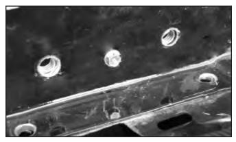
NOTE: This will secure the nut plate to the firewall, making future removal and reinstallation of the Strut Tower Brace significantly easier. The head of the sheet metal screw should line up with the hole at the back of the strut tower brace mounting pad.
