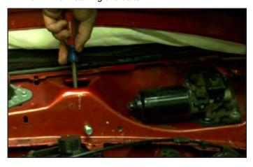
31. Install the #8 sheet metal screw into the small hole in the nut plate. Remove the 5/16"-18 bolts.
