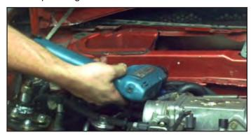
21. Drill the holes at the firewall. Start with a 1/8" pilot bit. Drill out to 5/16" and deburr the holes. Note: Hold the hood vertical when drilling downwards into the pinch weld. That will provide clearance for the drill motor. *Tip:* Hold the hood upright by using a rope or strap to tie the hood to the steering wheel.
