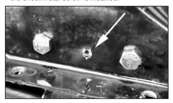
Tip: On the Driver's Side, tape the nut plate to a screwdriver to help hold it in position behind the firewall while installing the bolts.
