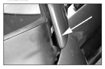
16. Remove the plastic cowl cover at the base of the windshield. It is held on with clips. Remove it by gently prying it upwards. When it is loose, disconnect the hose to the windshield washer nozzles (pointed to below).
