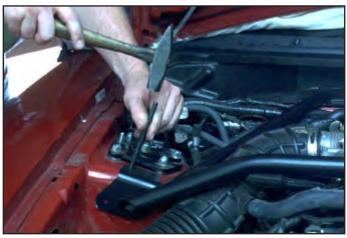
10. Center punch the mark. Drill a 1/8" pilot hole. Drill out to 5/16". Deburr the hole.
