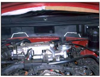
5. Remove the alarm siren (if so equipped) from the firewall. Then remove the plastic cover from the firewall. It is held on with several small sheet metal screws, as well as the hood seal.
