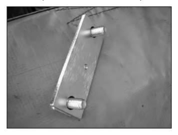
23. Line up the nut plate on the 5/16" holes drilled in the firewall in Step 20. Use the bolts installed in the previous step as guide pins. Make sure that the small hole in the plate is biased downward.
