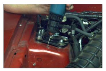
11. Set the Strut Tower Brace back into place. Insert a 5/16" bolt into the hole to hold the brace in position. Hold it both downwards and rearwards. Mark the positions of all of the other holes on both strut towers. Remove the Strut Tower Brace before drilling.
