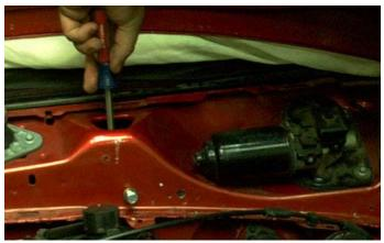
28. Install the #8 sheet metal screw into the small hole in the nutplate. Remove the 5/16"-18 bolts.
