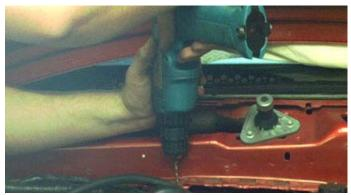
Install the 5/16"-18 x 3/4" long bolts in the nutplate. Thread them through so that they protrude on the flat side of the nutplate. It is not necessary to thread the bolts all the way in.
