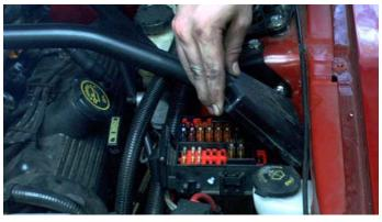
NOTE: If the fuse box cover cannot be opened, reposition the fuse box by moving it forward. This can easily be done by slipping a screwdriver between the front of the strut tower and the rear of the metal fuse box mounting tabs (these are attached to the strut tower). Gently pry the tabs forward. This will move the fuse box slightly forward.
