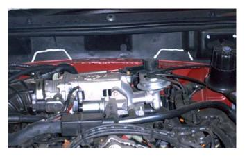
Remove the alarm siren (if so equipped) from the firewall. Remove the hood seal from the cowl. Then remove the plastic cover from the firewall. It is held on with several small sheet metal screws.
