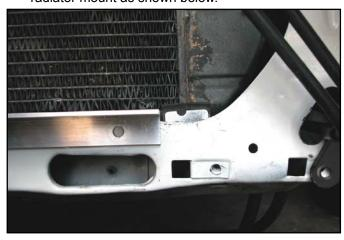
13. Using center punch, mark the center of one of the 5/16" L-bracket holes on lower radiator core support. To ensure accurate placement, *CAREFULLY* drill a pilot hole first, followed by a 11/32" drill bit. If necessary, use a file to de-burr the hole.
