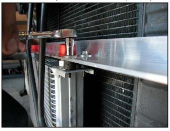
24. Push down on the upper L-bracket and oil cooler assembly to make sure it is fully seated on the lower vibration isolators. Vise Grip the upper L-bracket through the headlight opening.
