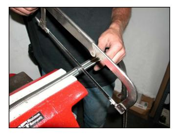
35. A 90° fitting and a straight fitting must be installed onto the ends of the cut hose. Disassemble the red socket from the blue nipple on one of the fittings. Use motor oil to lubricate the inside threads of the socket. Install the socket onto the hose by twisting the socket COUNTER-CLOCKWISE. Butt the end of the hose up to the base of the threads of the red socket.
