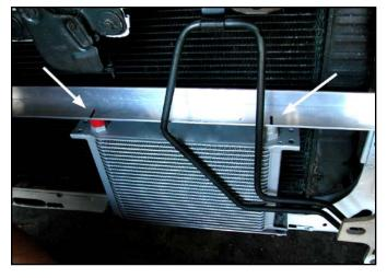
NOTE: Some modification may be required if you are using your stock power steering fluid cooler. If the upper L-bracket will not fit behind the power steering fluid cooler then bend the mounting tab towards the front of the car or use washers to shim the bracket forward.
