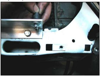
17. With oil cooler placed on vibration isolators, hold upper L-bracket against oil cooler outlets and mark the center of the fittings on the upper L-bracket. Make sure upper L-bracket is centered left-to-right on the car.
