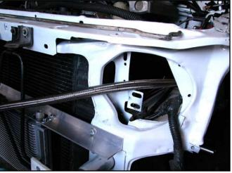
34. Once you have determined where you want to cut the hose, use masking or electrical tape to tightly wrap where you will be cutting. Squarely cut through the tape and hose with a sharp 32 teeth per inch hacksaw. Trim frayed ends of the hose with a sharp pair of metal snips and remove the tape.
