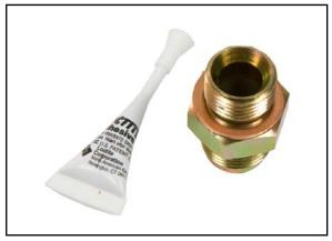
29b. If installing kit OC-2 (w/o thermostat), coat the tapered pipe threads of two AN to pipe fittings with Loctite Thread Sealant. DO NOT COAT FIRST THREAD.
