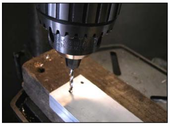
10. On the short leg of the L-bracket, mark a point 1.25" from each end and centered on the leg. Center punch your marks, drill with a 11/32" drill bit and de-burr.
