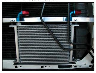
29a. If installing kit OC-2 (w/o thermostat) go to step 29b. If installing OC-1 (w/ thermostat), coat copper washer with Loctite Thread Sealant. Place washer over threads of adapter.
