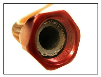
36. Use a felt pen to mark the hose at the base of the socket, so that you can tell if the hose is getting pushed out during the rest of the assembly.
