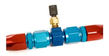
20. Reinstall the hose with the MM In-Line Temperature Sensor Kit onto your car, and check for leaks.
