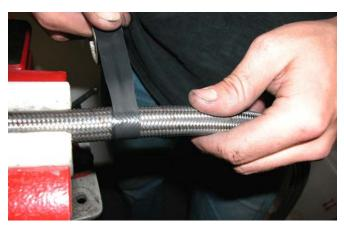
Squarely cut through the tape-wrapped sections of the hose using a sharp 32 TPI (or finer) hacksaw blade.
