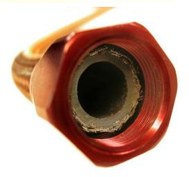
12. Use a felt pen to mark the hose at the base of the socket, so that you can tell if the hose is getting pushed out during the rest of the assembly.
