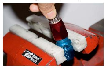
14. When you can no longer tighten the fitting by hand, clamp the socket in a vise (again, use soft jaws). Use an appropriate size wrench to tighten the nipple until the nipple is within 1/16" of bottoming on the socket.
