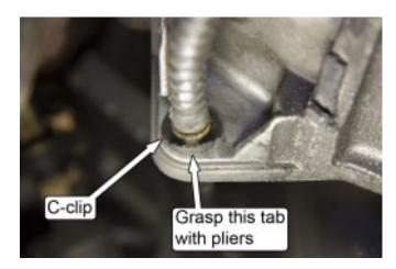
8. Unhook the inner cable from the clutch fork by pulling the end of the inner cable out of the smaller hole, then sliding it towards the transmission and out of the larger hole. Then carefully remove the cable from the vehicle by pulling it out from either the top or bottom of the car. Gently free the cable if it gets stuck or entangled. Do not attempt to force it out, as this can damage other components.
