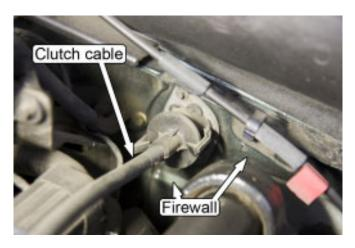
Remove the hex head bolt and bracket holding the cable to the unibody with the 5/16" socket and extension.
