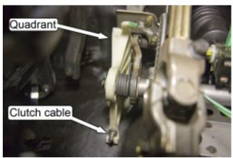
4. Open the hood and locate the clutch cable. It passes through the firewall high up on the driver's side, between the valve cover and the master cylinder. Remove the hex head screws that retain the cable with the 3/16" socket and extension.
