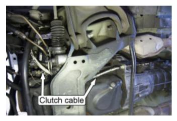
10. Feed the end of the new cable through the bellhousing and reinstall the C-clip removed in Step 7 onto the cable housing. Slide the end of the inner cable into the clutch fork, making sure that the end of the cable is properly seated at the very end of the clutch fork. To keep the inner cable in place during the remainder of the installation, wrap two turns of masking tape around the clutch fork just inboard of the inner cable.
