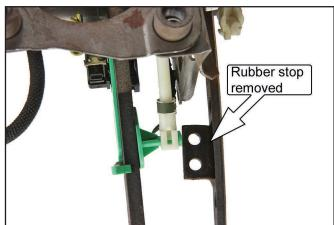
3. Place the Pedal Stop Nut Plate on the underside of the pedal stop bracket as shown below. The knurled bolt should be located in the lower hole of the pedal stop bracket.
