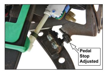
14. There is a clutch interlock switch located on the outboard side of the pedal box assembly that must be reset to allow the engine to crank. Locate the notched plastic shaft extending from the switch. On the shaft is a small plastic ring. With the clutch pedal up, slide the ring toward the switch housing until it touches.
