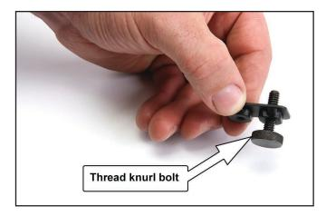
2. Remove the rubber pedal stop pad located on the clutch pedal.
