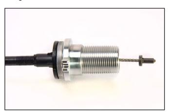
17. While holding the clutch cable housing in one hand, turn the knurled part of the Firewall Adjuster with the other hand. It should spin smoothly with some resistance.
