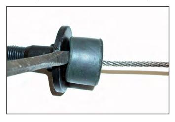
14. Lightly sand the casting flash in the recessed part of the cable housing until smooth.
