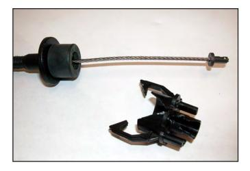
13. With a flat blade screw driver, pry the rubber bushing from the end of the cable housing.
