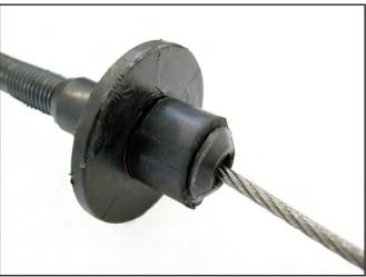
NOTE: Before installing in the car, you will need to check the operation of the Firewall Adjuster on the clutch cable.
