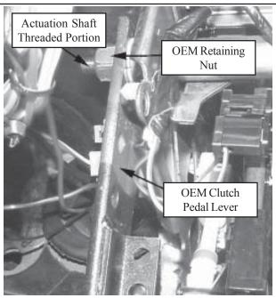
Dismount the OEM clutch pedal lever from the square shoulder of the actuation shaft such that the square-shaped hole in the OEM clutch pedal lever is completely off the threaded end of the actuation shaft. If necessary, remove the clip securing the OEM clutch pedal lever to the clutch lock-out switch. (See the following picture)
