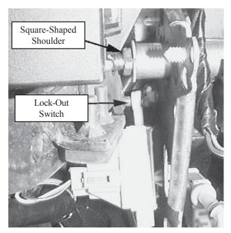
4. Position the MM clutch pedal adjuster on the actuation shaft with the square-shaped hole in the MM clutch pedal adjuster engaged with the square-shaped shoulder of the actuation shaft. The MM clutch pedal adjuster should be positioned such that it extends towards the floor of the car with the tapered edge of the MM clutch pedal adjuster facing the firewall. (See the following illustration)
