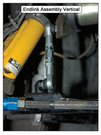
5. With the endlink assembly correctly oriented to position it as vertical as possible, secure the Mounting Block to the control arm by tightening the M10-1.5 x 16mm long bolt to 33 lb-ft. The mounting block must be rotated to aid in making the endlink vertical.
