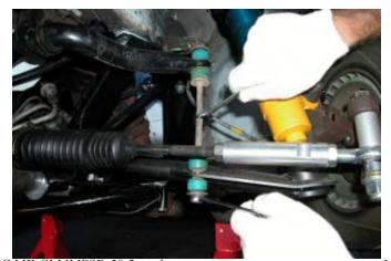
Remove the four bolts which hold the swaybar pivot U-brackets to the chassis. Hold the swaybar while removing the bolts to prevent it from falling.
