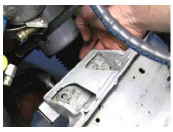
10. Liberally grease the inside of the universal front sway bar bushings with the supplied Prothane Super Grease. Coat 100% of the bushing surface in contact with the swaybar.
