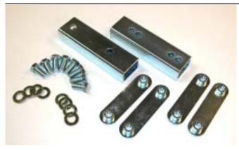
The MM Front Swaybar Relocation Kit allows the option of moving the front swaybar forward 0.6" or 1.1". This keeps the swaybar endlinks in alignment with the control arms when the front wheels have been moved forward with an MM K-member and MM Forward Offset Control Arms. The MM Front Swaybar Relocation Kit can also be used with other aftermarket K-members that move the wheels forward. The use of this kit requires a set of universal swaybar U-brackets (P/N 6-1124 to 6-1137)
