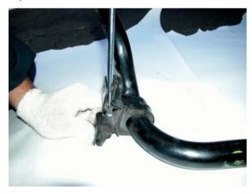
Remove rubber swaybar pivot bushings from the swaybar.
