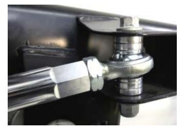
Note: MM recommends a spacer stack that is centered (2 below, 2 above) as a starting inner-spacer configuration for **2003-04 IRS** cars. Place the OEM Spacer on the **top** of the MM spacer stack (OEM Spacer not shown in photo).
