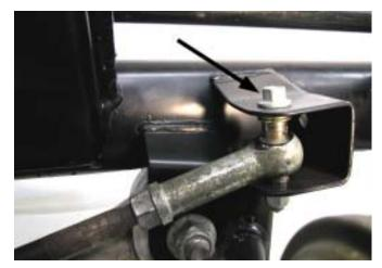
Note: 2003-04 cars have a factory spacer installed between the upper mounting tab and the tie-rod end crush sleeve. Keep this part. It will be re-used.
