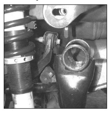
Apply a thin layer of the supplied grease on the interior surface of each shell and to the exterior surface of two MM Polyurethane IRS Subframe Bushings.
