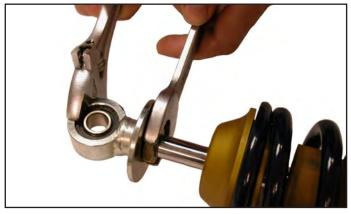
20. Insert two bearing inserts into the lower rod-end of the shock.
