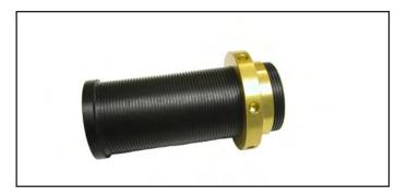
14. Install a MM threaded sleeve onto each shock body by sliding the sleeve on from the top end of the shock, with the flanged lip of the threaded sleeve facing downward. There should be a circlip in the second groove from the bottom of the shock. The threaded sleeve will completely encapsulate this circlip and prevent it from dislodging from the shock.
