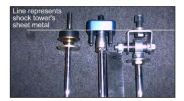
NOTE: The installation of the upper shock mount is not easily reversible. Due to the drilled holes, the shock tower will be too weak if the shock is run in stock configuration without welding the holes closed.
