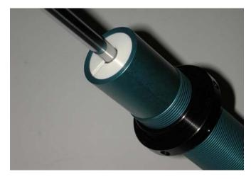
15. Place one of the bumpstops into position on the shock shaft.
