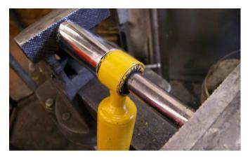
10. Use a similar process to remove the rubber bushings from each shock eyelet. Select a socket that is large enough to accept the rubber bushing into it's center, but will still support the steel eye of the lower shock mount. Then select a smaller deep socket that will be able to push the rubber bushing out of the steel eye.
