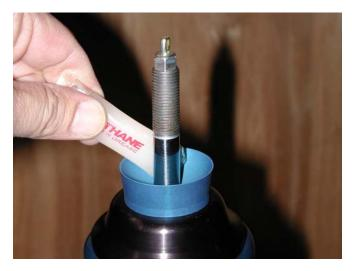
22. Place one of the Delrin pivot balls on the shock shaft with the curved side facing down toward the aluminum pivot socket.
