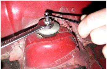
29. Raise the lower spring perch until the spring is just contacting the upper and lower spring perches.
