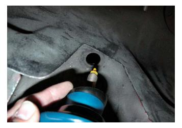
28. From inside the car, on top of the shock tower, place a Koni rubber isolator, thrust washer, and nut on top of
