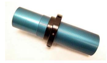
14. Install the threaded sleeve onto the shock absorber body by sliding the sleeve down from the top (piston rod) end of the shock, with the flanged lip of the sleeve towards the stud. Slide the sleeve downward until the lip of the threaded sleeve firmly contacts the upper portion of the shock body. Reinstall the bump stop shim so that it seats squarely against the top of the shock.
