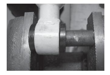
18. Place one of the coil-over springs onto the lower spring perch. Position the lower spring perch so the top of the spring is well below the top of the step in the shock shaft. This will make the installation of the remaining parts easier.
