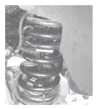
6. From inside the car, remove the nut, thrust washer and upper rubber isolator from the top of each shock shaft. Save these three components, as they will be re-used later in the coil-over installation.
