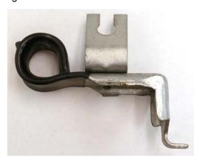
15. Slide the Parking Brake Cable Bracket back onto the parking brake cable and reattach the parking brake cable to the caliper.
