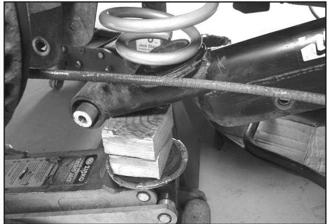
9. Remove the control arm pivot bolt from the chassis and remove the control arm from the car.
