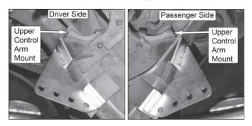
NOTE: Check for interference between the passenger side Chassis Mount and the fuel line. Along the inside of the frame rail there is a small clip holding the fuel line to the frame rail which may need to be removed.
