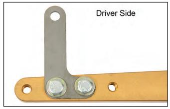
21. Bolt each Chassis Mount to the inside of the Installation Plate as shown. These brackets are specific to the driver and passenger sides. Make sure the two 5/16" holes in the U-bracket are facing outboard. Use (2) 3/8" X 1" bolts and (2) 3/8" AN washer, placing one washer under the head of each bolt. Snug the bolts just tight enough so that the brackets can still be pivoted, although with some effort.
