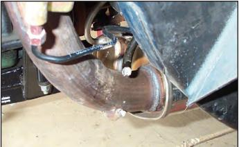
28. It is recommended that the exhaust hanger chassis brackets are removed from the vehicle and trimmed further. Cut off the unnecessary portion of the Exhaust Hanger Chassis Brackets as shown below.
