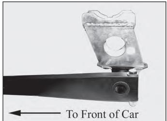
23. Place a jack stand or blocks of wood just to the rear of, and approximately level with, the bottom of the differential. Rest the Swaybar on the jack stand or wood with the arms facing forward.
