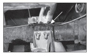
51. Remove the Installation Plates.
