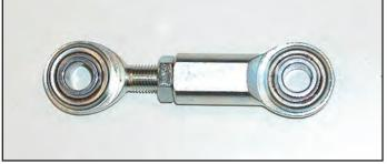
59. It is recommended that you start with the bar in the fullsoft setting (forward holes) and increase the stiffness if you find it necessary. Bolt the Female end of the rod-end assembly to the outboard side of the flange on the Chassis Bracket using parts in the following order: Under the head of a 3/8" X 1 1/2" G5 bolt, place (1) 3/8" AN washer, the Female Rod-End then (3) 3/8" AN washers. Thread the bolt into the Chassis Bracket and torque to 33 ft-lb.
