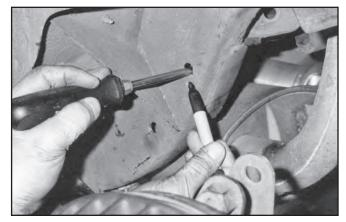
Transfer each measurement to the appropriate tube and cut the tube 1/16" to 1/10" shorter than your mark. That gives a slight "crush" to the frame rail when the bolts are tightened and ensures the mount will be secure when installed. Be sure to label each insert for the right and left side of the car, and which end is toward the front or rear. Do not be surprised if every tube is cut to a different length.
