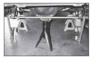
24. Mate the Axle Mounts to the axle; their exact position at this time is not critical. As you do so, slide a U-bolt into place on each Axle Mount. Be careful to not pinch the brake lines. Thread (8) 3/8" Nylock Nuts onto the U-Bolts, placing one 3/8" Grade 8 washer under each nut. Leave the brackets slightly loose so they can pivot on the axle tubes. NEVER weld the Axle Mounts to the axle! Welding on the axle will cause the axle to warp!
