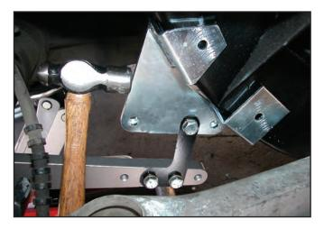
The proper position for the Chassis Mount is with it completely touching the bottom of the rear subframe, and the inside of the upper bracket will be touching the horizontal portion of the upper control arm mount.
