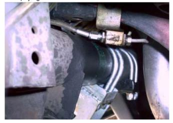
If you wish to lower your car more than 2" for racing, you will need additional bump travel to avoid excessive bottoming of the suspension. With modifications, the MM Upper Racing Shock mount will allow more bump travel than stock, but first you must re-route the brake lines to avoid potential interference. If you are unsure of your abilities to re-route brake lines, take your car to a professional race preparation shop. Typical brake repair shops will not be able to help you.
