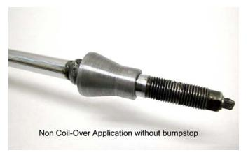
20. Place a Shock Shaft Reducer onto the shock shaft with the larger diameter on the bottom.
