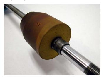
17. For non coil-over applications with bumpstops, place a 9/16" flat washer over the shock shaft and on top of the bumpstop. If you are not using a bumpstop you will not need to install this washer. Skip to step 19.
