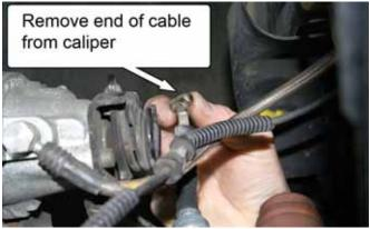
4. Slide the parking brake cable out of the slot in the OEM control arm.
