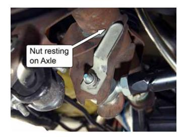
11. Install the NEW captive nut into the chassis mount location. The rearward tab slides into the slot first, then the frontward tab is lowered into a channel.
