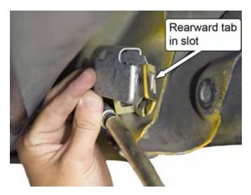
12. Swing the chassis-end of the arm in place at the front chassis mount. Secure it with one of the provided, shorter mounting bolts.
