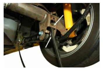
13. Torque the control arm mounting bolts to 129 ft-lb.
