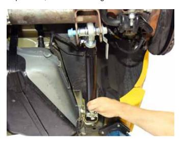
NOTE: The axle may shift slightly when the OEM control arm is removed. If necessary, you may use a pry bar to shift the axle into position to align the arm with the mounting hole. Place the end of the pry bar in the control arm mount and push the pry bar against the end of the control arm to move it.
