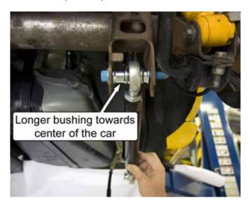
10. Install the provided OEM captive nut on the rear control arm mounting bolt, and snug the bolt. Allow the metal flag on the captive nut to rotate up against the axle bracket. It is intended to act as a back wrench for bolt tightening.
