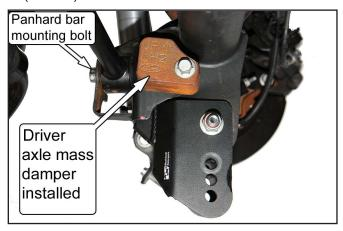
34. Torque the Panhard Bar mounting bolt first, then the 2 side bolts from Step 31. Torque all three bolts to 175 Nm (129 lb-ft).
