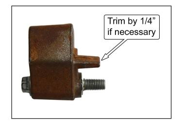
33. If reinstalling the axle mass damper, do so at this time and torque the mounting bolt to 90 Nm (67 lb-ft).
