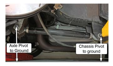
C. Measure the distance from the ground to center of the passenger side rear lower control arm mounting bolts. These measurements will be used to determine the correct mounting hole position to use on the relocation brackets.
