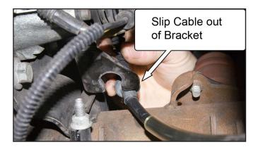
10. Unhook the parking brake cable end from the caliper.
