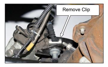
9. Pull down on the end of the parking brake cable housing and slide it rearward until it disconnects from the brake caliper.
