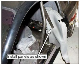
59. Pass the seat belts up through the mounting slots in the quarter panels and hang them over the inboard edge.
