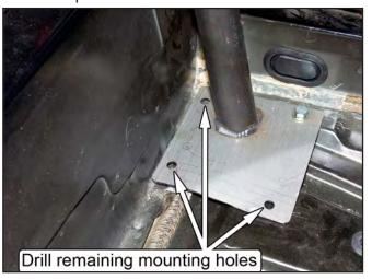
28. Mark the position of the four mounting holes in each rear support mounting pad onto the wheel well using a center punch.
