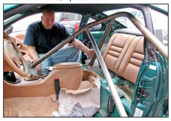
47. Keep the roll bar as low to the ground as possible in order to keep adequate clearance on the upper door frame.
