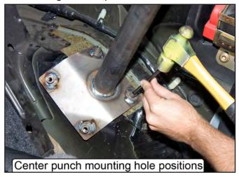
29. Move the main hoop forward and drill the four holes marked on each wheel well to a 7/16" diameter. Use 1/8" diameter pilot drill to start the holes.
