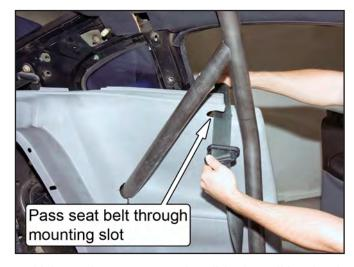
60. Using at least two people, slide the roll bar back into its final mounting position. As the roll bar is moved back, the lower plastic quarter panels must be gently forced over the rear seat bulkhead into their original mounting position.
