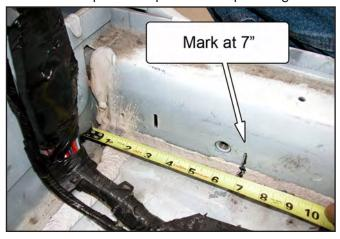
17. Again, starting at the rear corner of the driverside floor pan, make a mark 7" inward from the corner, along the rear bulkhead. Repeat for the passenger side.
