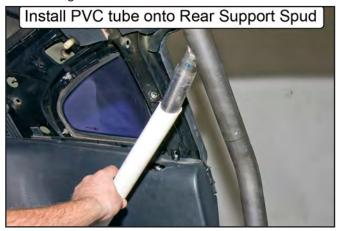
35. Slide the angled end of the PVC tube down against the quarter panel. Rotate the PVC tube so the end is parallel to the face of the panel and mark the panel around the outside of the tube.
