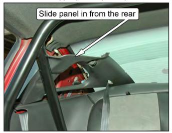
**NOTE:** Each panel has a long plastic guide pin located near the front and rear of the panel. Make sure these pins are inserted into their respective mounting holes in the sheet metal for proper installation.
