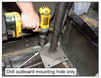
27. Drill the three remaining holes in each of the main hoop mounting plates. It will be necessary to mark the outboard hole and temporarily move the hoop to allow access for the drill.
