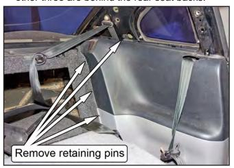
13. Remove the lower plastic quarter panels by pulling forward on the B-pillar edge. Once the panels unsnap, angle them out and over the rear seat bulkhead.
