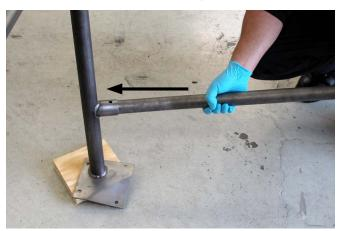
3. Rotate the door bar so that the Mounting Pad sits flush on the floor of the car.
