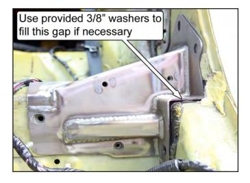
20. Check the gap between the bracket and the vehicle at H8. Use the provided 3/8" G8 washers to close the gap to 1/8" or less. When satisfied, insert one of the factory mounting bolts into the hole to prevent the washers from being dislodged.
