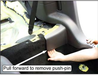
Remove both front plastic kick panels. Pull the portion closest to the firewall inboard to disengage the push-pin retainer, and then pull the panels rearward.
