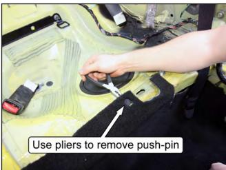
14. Pull the driver and passenger sides of the carpet up and fold them over the center console to protect it during the remaining installation. Use the provided zip-tie to hold the two halves of the carpet together.
