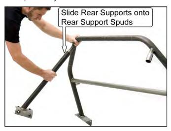
26. Place the roll bar into the vehicle by tilting the hoop forward and passing it through the passenger-side door. Once the roll bar is in the vehicle, tilt it rearward and place it onto the MM support brackets and the rear support mounting pads on the inner corner of each rear wheel well.
