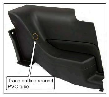
53. Remove the rear half of the plastic panel from the vehicle and hole saw through the location marked for the rear support. Use a 2" hole saw if available, or a 1-3/4" hole saw can be used and the opening can be filed out larger.
