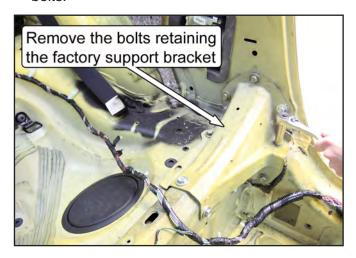
17. Scrape away any excess seam sealer around the factory support bracket mounting area.
