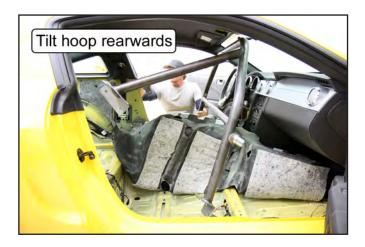
27. Trace an outline of the rear support mounting pads onto the driver- and passenger-side wheel well, and then remove the roll bar.
