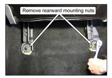
3. Slide the seats all the way back to remove the two front hex bolts using a 13mm socket.
