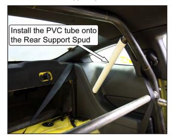
51. Set the roll bar back in its mounting position and slide the PVC template down until it contacts the plastic quarter panel. Rotate the PVC tube so the end is parallel to the face of the panel.
