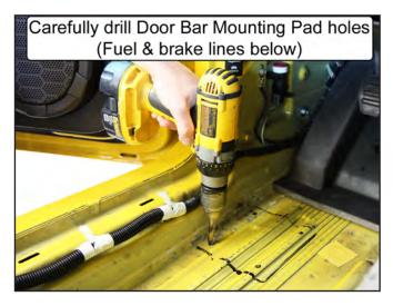
**NOTE:** There ARE fuel and brake lines directly beneath the driver-side door bar mounting pad. Place the door bar doubler plate between the underside of the floor pan and the lines as a shield when drilling to prevent punctures.
