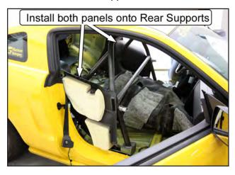
71. Lift the roll bar, along with the plastic panels, into position.
