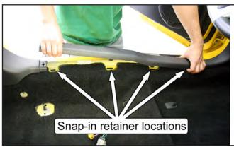
11. Remove the rear quarter panels. There are three push-pin retainers on each panel; one is located at the front of the seat bulkhead and two are at the rear seat backrest. Carefully pull the rear half of the panels inwards to disengage the snap-in retainers located below the quarter window, and then pull the panels forward.
