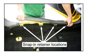
Remove both front plastic kick panels. Pull the portion closest to the firewall inboard to disengage the push-pin retainer, and then pull the panels rearward.
