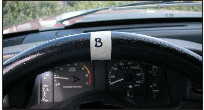
22. Divide the number of turns required to go from full lock to full lock in Step 20, by 2.
