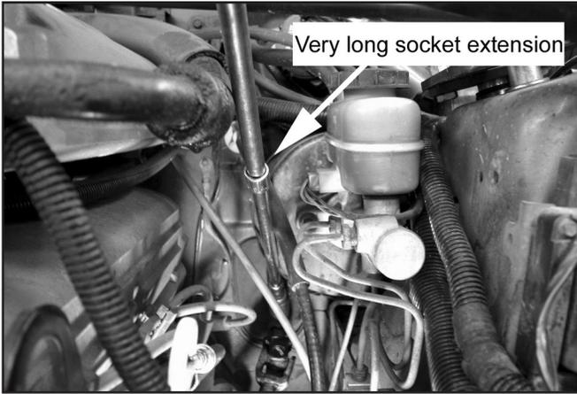
3. Disconnect the steering shaft from the steering rack input shaft by removing the pinch bolt.
