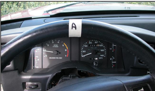
20. Rotate the steering wheel counter-clockwise until full lock is reached. For future reference (in Step 21), count the number of turns required to turn the steering wheel from full lock to full lock.
