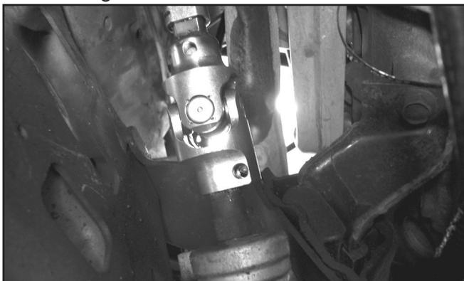
*NOTE: The groove is a safety feature that prevents the U-joint from pulling off the steering rack input shaft in the event of the installed pinch bolt coming loose.*
