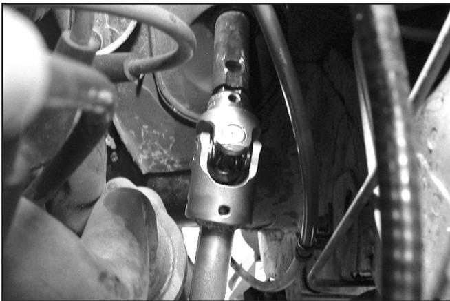
11. Once the bolt holes are aligned, insert the original retaining bolt and nut. The bolt will be torqued at a later step.
