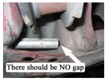
Remove the steering rack mounting sleeves from the k-member. Mark each sleeve as to which side of the vehicle they were removed from.
