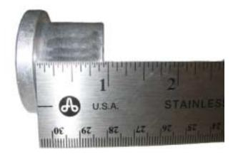
13. After ensuring that they are short enough, reinstall both aluminum rack bushings into the front of the rack.
