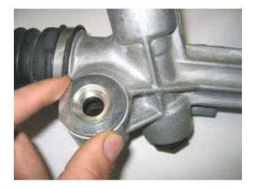
NOTE: Older revisions of the aluminum rack bushings offered by MM (and some of our competitors' bushings) are too long to properly work with the MMST-7.1 upgrade kit without some minor trimming. Use the following procedure to check and modify your aluminum rack bushings.
