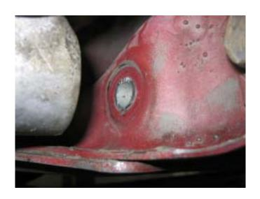
10. Place the rear half of the MM aluminum rack bushings (with the machined concave mounting face) in the rearward side of the steering rack mounting holes.
