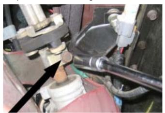
Remove the two nuts and washers holding the steering rack to the k-member.
