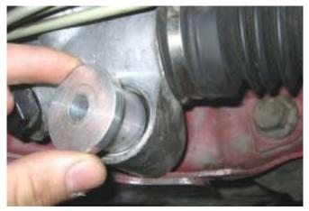
18. Slide the steering rack mounting bolts completely forward and install one of the supplied Yellow G8 washers on each bolt.
