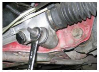
4. Remove the two steering rack mounting bolts.
