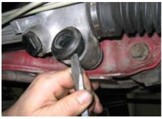
Remove the steering rack mounting sleeves from the k-member. Mark each sleeve as to which side of the vehicle they were removed from.
