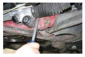
NOTE: It may require considerable force to pull the rack forward from the k-member. We recommend placing a small pry bar or large screwdriver between the rack housing and k-member to pull the rack forward. Because the rack must be pulled free from both sleeves at the same time, the rack must be pulled evenly. Be careful not to damage the power steering lines.
