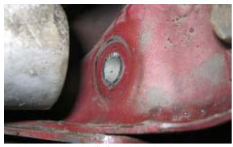
12. Place the rear half of the MM aluminum rack bushings (with the machined concave mounting face) in the rearward side of the steering rack mounting holes.
