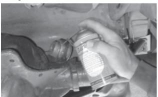
4. Liberally apply anti-seize compound to the threads of the 7/16"-20 x 5" Grade 8 bolt supplied.
