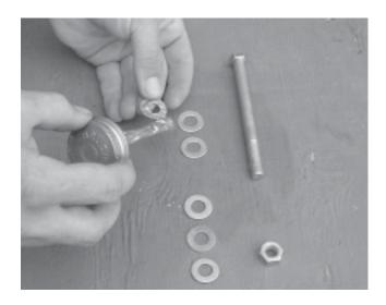
5. Slide three 7/16" Grade 8 washers onto the bolt. Slide the 7/16" bolt through the hole of the Bushing Removal Cup (the larger of the two cups). Place the bolt and the cup over the flanged end of the control arm bushing in the differential.
