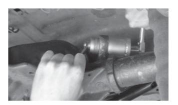
9. When the bushing is almost out of the differential, care must be taken to make sure that the 1-3/4" x 3/8" disc is alligned and can pass freely through the hole in the differential housing.
