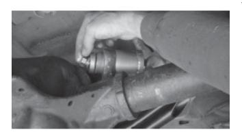
8. Tighten the 7/16" Grade 8 bolt and nut to draw the bushing out of the differential.
