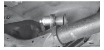
drawing the bushing into the differential.
