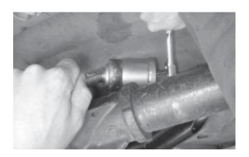
The bushing, when extracted from the differential housing, will end up inside of the Bushing Removal Cup.
