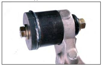
12. Using a pair of wrenches, tighten the bolt to pull the cross-axis joint into the Removal Cup.
