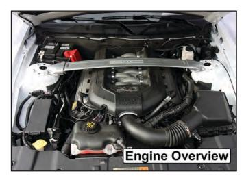
1. If not already done, remove the two upper engine isolator nuts using a deep 15mm socket (one on each side of car).
