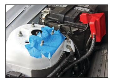
5. Assemble the two halves of the engine support beam and place the mounting pads over the inboard studs of the upper strut mount. The beam is telescopic to accommodate variations in strut tower widths.
