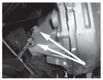
27. Remove the two mounting bolts that secure the forward differential mounting flanges to the IRS subframe, along with the vibration damper and stock bushings.
