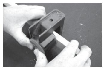
52. Install the Rear differential mount on the IRS Subframe. Do not torque. The differential mount should be snug, but still able to rotate with little effort.
