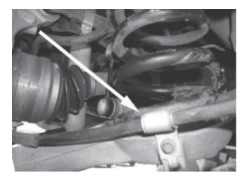
5. Make sure the parking brake is not set, and then remove the parking brake cable housing retaining clip on each caliper.
