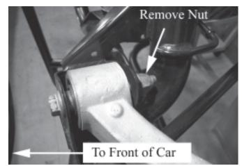
31. Remove the two mounting bolts that secure the forward differential mounting flanges to the IRS subframe.
