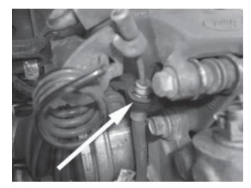
6. Disconnect the parking brake cable from the parking brake lever on each caliper. Remove the cable from the locating hole in the calipers.
