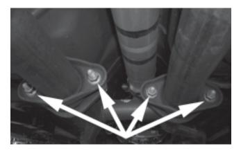
4. Unbolt the parking brake cable mounting-bracket from each control arm.
