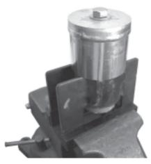
45. Use a socket and a wrench to tighten the nut & bolt assembly until the nut just bottoms on the bolt threads. It does not take much effort, so do not over tighten.
