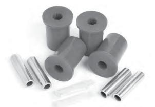
Improve handling and reduce wheel hop with MM's urethane IRS subframe bushings. Replacing the stock rubber mounting bushings with urethane virtually eliminates movement of the IRS subframe relative to the chassis.
