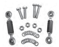
The MM endlinks allow adjustment to eliminate the swaybar preload that occurs when one of the endlinks is not exactly the correct length for a particular installation. The swaybar twists and becomes preloaded if the endlink length is off by even a very small amount. The preload will alter the car's corner weights, which in turn causes asymmetrical handling characteristics.
