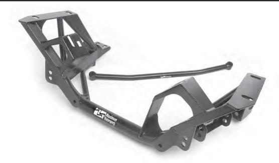
Get more front grip and dramatically improve handling with the optimized suspension geometry of a Maximum Motorsports Tubular K-member. At only 37 lbs., the MM K-member is 26% lighter than the original and the strongest, stiffest, and most durable K-member available. Installing the MM Tubular K-member reduces weight and greatly improves cornering ability.
