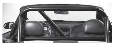
MM Roll Bar with diagonal brace installed
