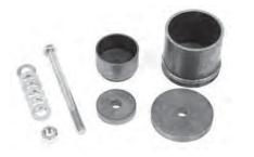
This tool from MM makes it much easier to change the stock rear upper control arm bushings at the differential (Part E4SZ-5A bushings). The bushings are a press fit in the differential housing, and are difficult to access. They're especially difficult to change if you're trying to do so without removing the rear axle assembly from your car. MM's unique tool makes this tough job much easier and faster.
