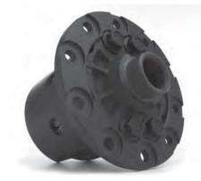
During braking there's little or no torque being conveyed to the differential, so there's little or no torque difference between the two rear tires. Therefore, the Torsen differential will not support any appreciable torque "wind-up" between the two rear tires during braking. For that reason the Torsen differential does not interfere with the functioning of anti-lock brake systems.
