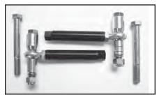
Commonly called bumpsteer kits, these adjustable outer tierod ends eliminate bumpsteer. Correcting excessive bumpsteer will offer sure-footed steering characteristics and require fewer
