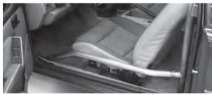
MM Roll Bar with low-slung door bars installed
