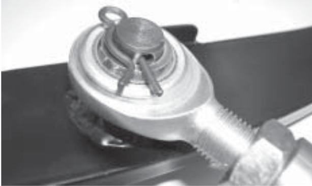
22. Fully thread the pushrod onto the rod end as a preliminary starting point for final brake pedal positioning (Step 46).
