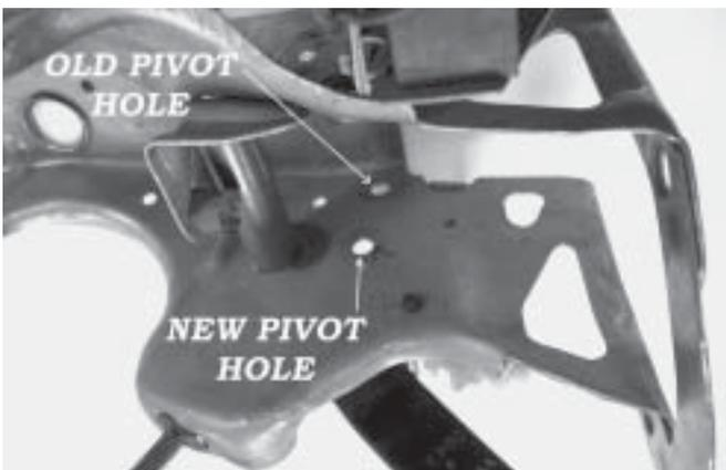
25. Mount the MM Pedal Arm in this lower pair of holes, re-using the OEM pivot bolt & nut.
