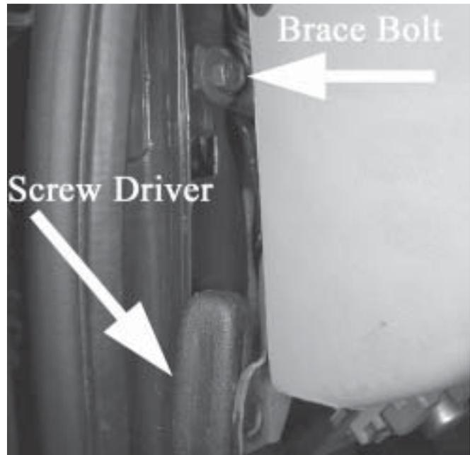
7. Disconnect the pushrod from the stock brake pedal. Save the OEM retaining clip for later use in Step 21.
