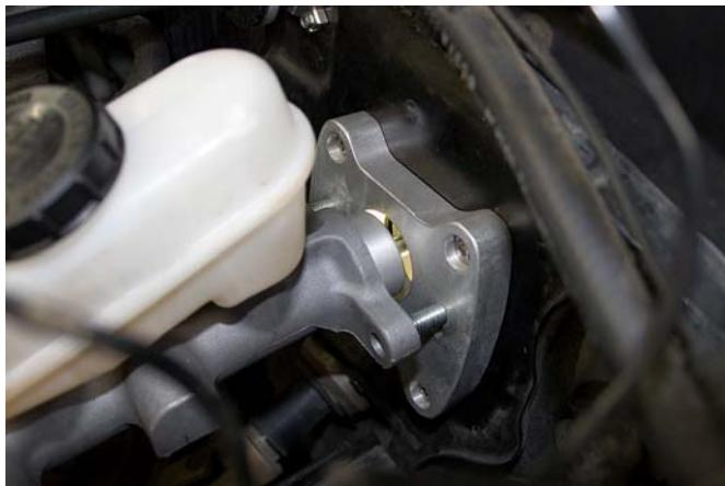
37. Place a 3/8" AN washer over each of the master cylinder mounting studs.
