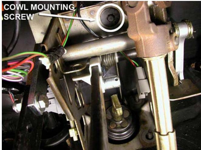
17. Remove the pedal box by rotating counterclockwise about the steering column. Be careful not to snag any electrical components as you remove the pedal box.
