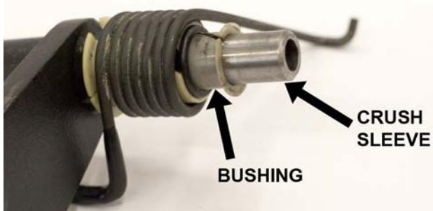
21. The pedal box requires a slight modification to relocate the OE torsion spring mounting hole from the tab in the middle of the pedal box to the passenger side face of the pedal box. To do so, drill a 5/16" hole in the passenger side face of the pedal box 1" down from the top of the firewall plate and 3/4" above it. When viewing the pedal box from the passenger side, the newly drilled hole should be on the same axis as the original OE spring mounting hole.
