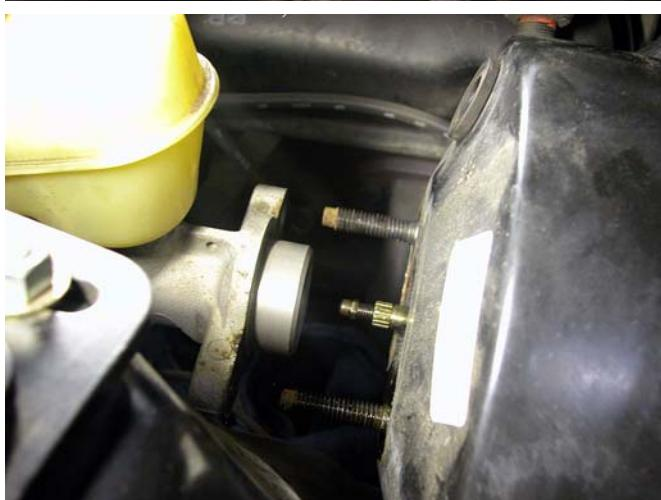
6. Cover any exposed brake lines or ports to avoid getting contaminants in the brake system.
