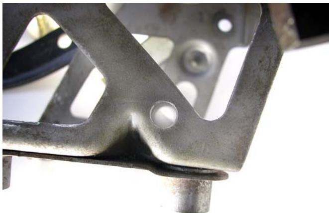
22. Install the MM Brake Pedal Arm in the pedal box by first hooking the long leg of the torsion spring in the hole drilled in the previous step. Line up the original pivot mounting holes with the MM Brake Pedal Arm pivot tube, and slide the OE pivot bolt through and secure with the OE nut.
