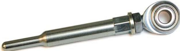
34. Slide the spherical rod end of the MM Brake Pushrod Assembly over the mounting stud on the MM Brake Pedal Arm while making sure that the other end passes through the firewall and MM Master Cylinder Adapter Block.
