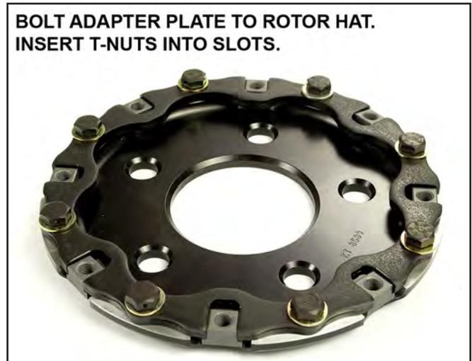
9. Torque the hex bolts to **180 in-lbs (15 ft-lbs)**. Tech tip: torque bolts in a star pattern (e.g. as you would with lug nuts) for even clamp loading.
