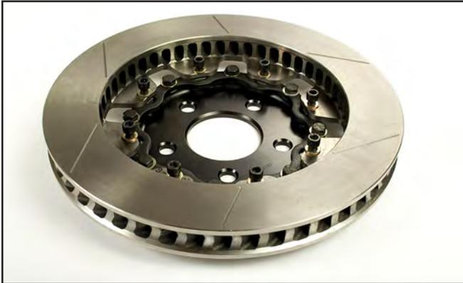
11. Torque the cap screws to **228 in-lbs (19 ft-lbs)**. Use the same star pattern when tightening the cap screws.
