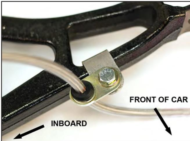
47. Temporarily mount the wheel and tire, and ensure that the hose is not rubbing against anything. If the braided stainless steel brake hose is in contact with anything, the hose will be worn through. If there is contact, reposition the MM IRS Control Arm Bracket on the control arm, or bend the MM Frame Rail Bracket to gain proper clearance.
