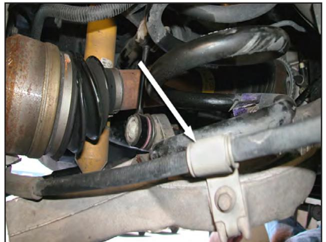
19. Pull the parking brake cable out of its spindle mount and guide hole.
