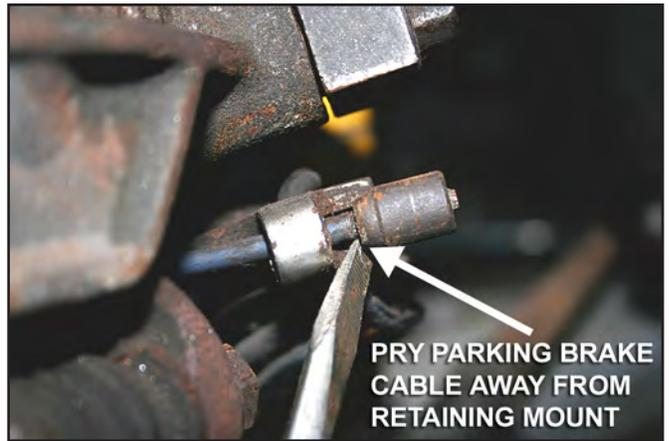
17. Remove the parking brake cable retaining clip.
