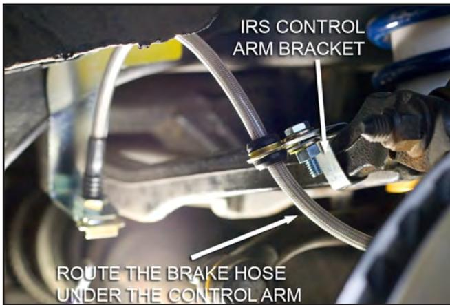
NOTE: Mounting the metal brake hose mount parallel to the control arm with the brake hose on the inboard side should provide adequate clearance to prevent the brake hose from contacting anything.
