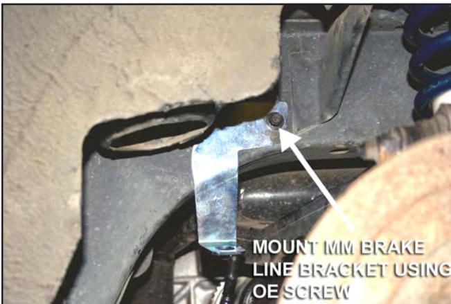
42. Connect one of the supplied braided stainless steel brake hoses to the MM Frame Rail Bracket by placing the 10 mm bubble flare fitting on the brake hose into the MM Frame Rail Bracket mounting hole.
