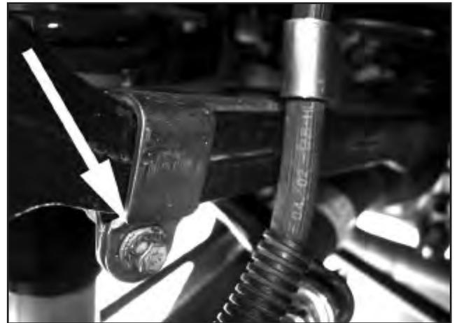
24. Unbolt the two (2) caliper mounting bolts. Save the mounting bolts for Step 26.
