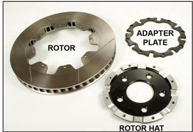
7. Inspect the floating rotor hat adapters and note the "HUB SIDE" text on one side of the adapter. This side should face the hub (inboard) when installed.
