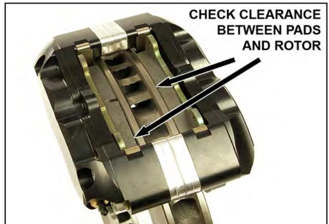
38. If there are no issues, torque the Wilwood caliper mounting bolts and spindle mounting bolts to **76 ft-lbs**.
