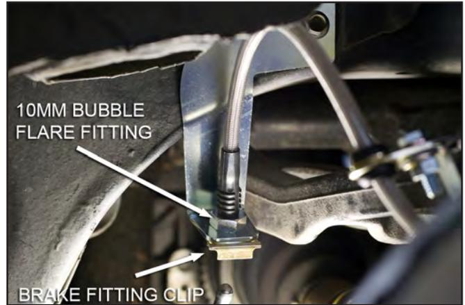
44. Route the braided stainless steel brake hose under the upper control arm and connect it to the -3 AN adapter fitting on the backside of the Wilwood caliper. Make sure the adapter fitting on the back of the caliper doesn't move while you are tightening the brake hose fitting. Tighten the fitting until it is snug.
