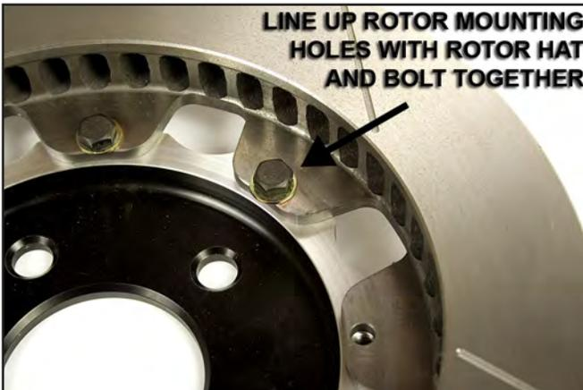
3. Torque the bolts to **180 in-lbs (15 ft-lbs)**. Tech tip: torque bolts in a star pattern (e.g. as you would with lug nuts) for even clamp loading.
