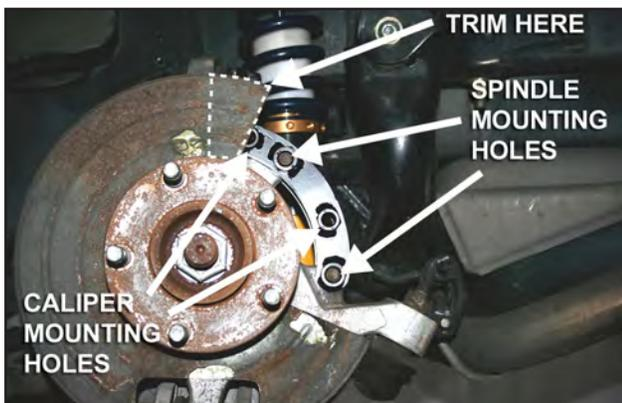
27. If trimming is necessary, unbolt the two (2) mounting bolts [older spindles have three (3) bolts] and remove the dust shield. Use appropriate cutting tools and safety precautions to trim the dust shield as necessary.
