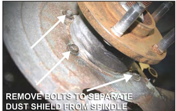
28. Reinstall the dust shield and torque the bolts to **89 in-lbs (7.5 ft-lbs)**.
