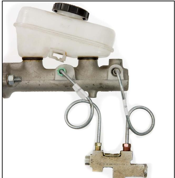
11. Tighten the ends of the brake hard lines to 12-16 ft-lbs at the master cylinder and the proportioning valve.
