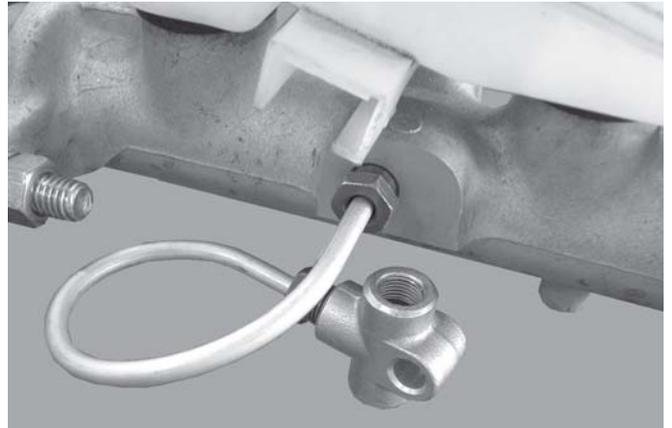
15. With flare wrenches, firmly tighten the fittings on both ends of the supplied brake line. Hold the T-Fitting with a crescent wrench to prevent bending the brake line.
