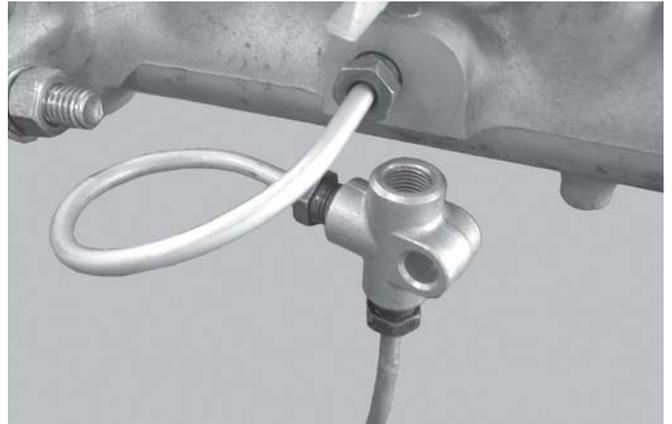
17. Thread the supplied brake line into the rear port on the factory proportioning valve and the top port on the T-Fitting. Firmly tighten both brake line fittings with a flare wrench. Hold the T-Fitting with a crescent wrench to prevent bending the brake lines.
