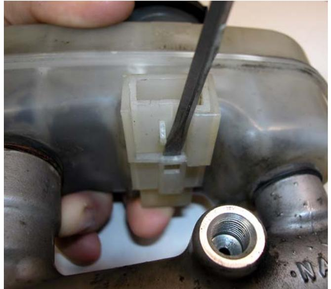
8. Install the low fluid level sensor into the new master cylinder by pressing in until it clicks into place.
