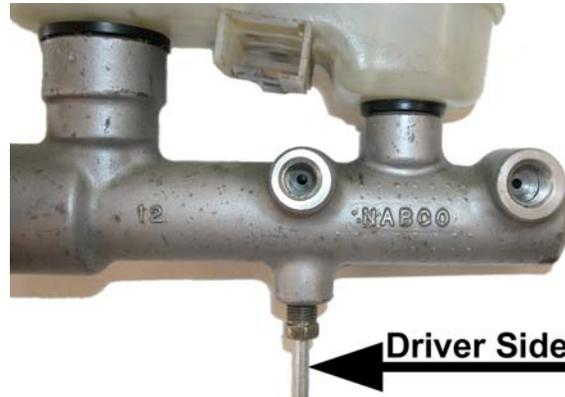
4. Thread the M10-1.0 bubble flare end of the supplied 3/16" brake hard line into the rear, side port of the stock master cylinder. Position the free end of the brake hard line above the stock proportioning valve.
