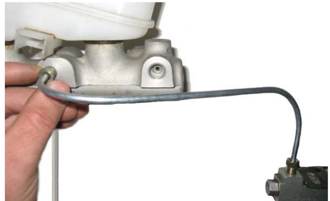
NOTE: The metric "bubble flare" can be differentiated from the standard "inverted flare" by a flare that extends past the threaded end of the fitting.
