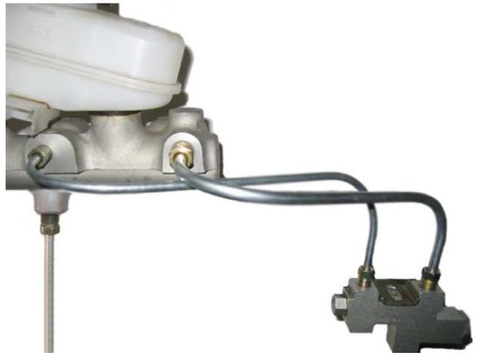
8. Tighten the ends of the brake hard line that connect the forward port of the master cylinder to the forward port of the stock proportioning valve to 12-16 ft-lbs.
