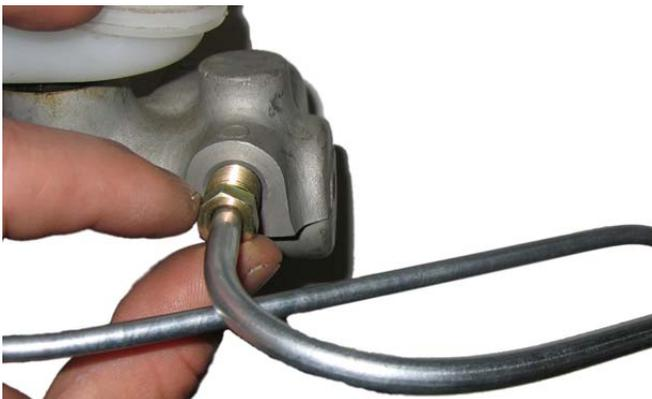
7. Thread the opposite end of the brake hard line installed in Step 6 into the forward port of the stock proportioning valve.
